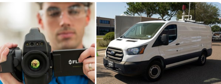
Optical gas imaging cameras detect leaks and reduce emissions.
