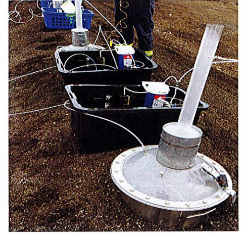
Sampling from a surface at a composting facility
